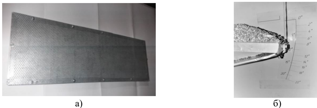
Figure 4 – Gas distribution grate: a – general view; b – grate inclination adjustment scale.
