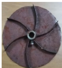
Figure 4. Accelerating disk of the impact centrifugal crusher
