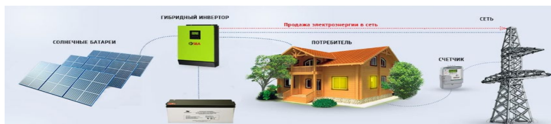
Figure 3 - Hybrid solar power plants
