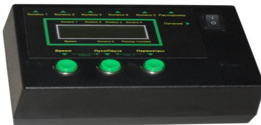
Figure 2: Six-channel pulse counter
